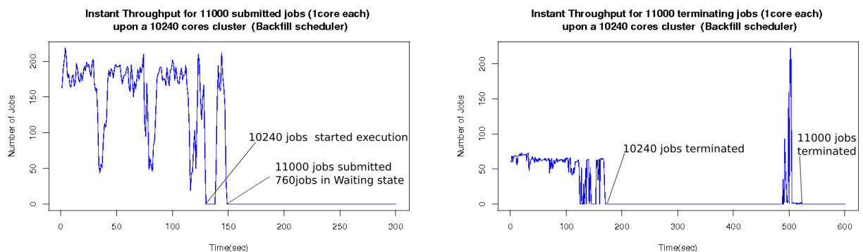
Figure 3.19: Throughput for submission(left) and termination(right) of jobs with SLURM - Backfill scheduler
