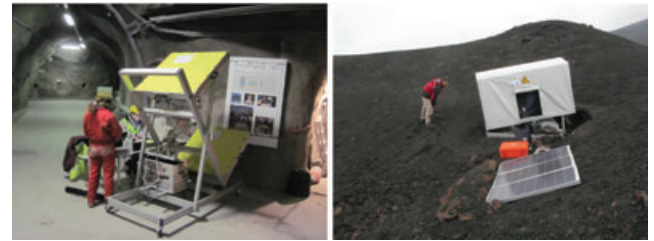
Figure 5. Top: general sketch of a small-size telescope. Bottom left: small-size telescope in operation in the Mont Terri underground laboratory. This telescope is equipped with two 16 \times 16 matrices with 5^2 \text{ cm}^2 pixels separated by D = 120 cm for this setup. Middle: sketch of the electronic mother board. Bottom right: another telescope, equipped with its protective tarpaulin and powered by solar panels, in operation near the South-East crater of Etna (Sicily) at an altitude of 3000 m.
