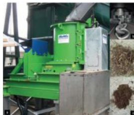
Figure 14 : Example of mechanical pretreatment unit called «Querstromzspanner»
