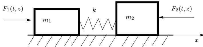
Figure 6.1: A mechanical system with Coulomb's friction.
